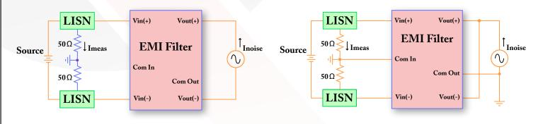
Figure B: Differential-Mode Current Attenuation, Imeas / Inoise
