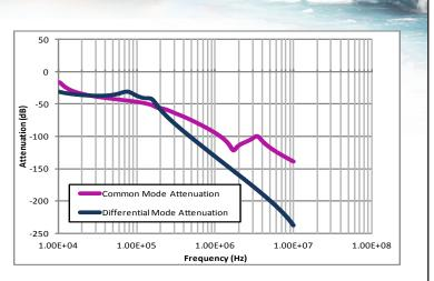
**Figure A:** Simulation of calculated common-mode and differential-mode current attenuation. The curves plot the ratio of noise current through a 50 $\Omega$  LISN sensing resistor to a noise source at the filter output (see Figures B and C).
